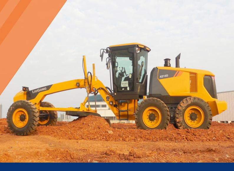
EngineCummins 6LTAA9.3Rated Power162 kW (217 hp / 220 ps) @ 2,200 rpmBlade Width4,270 mmMaximum Speed42 km/hDraw Bar Pull85 kNOperating Weight16,500 kg
