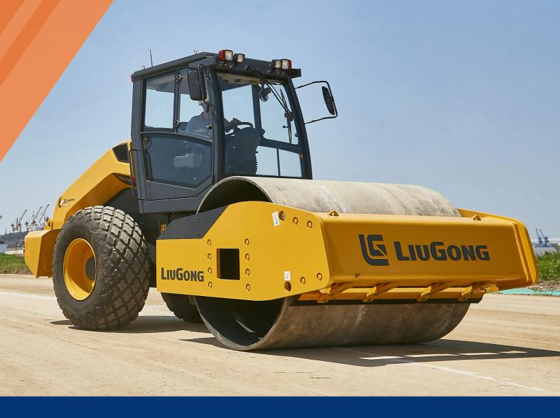
EngineCummins 6BTAA5.9Rated Power118 kW (158 hp / 160 ps) @ 2,200 rpmNominal Amplitude Range2.0 / 1.1 mmVibration Frequency Range30 / 33 HzCentrifugal Force Range300 / 190 kNWorking Width2,130 mmOperating Mass12,200 kg
