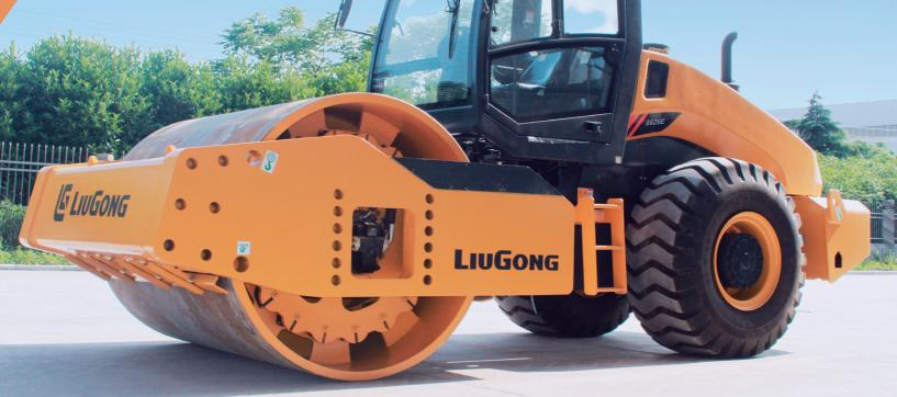
EngineShangchai SC9DK240G3Rated Power177kW (237 hp / 240 ps) @ 2,200 rpmNominal Amplitude Range2.0 / 1.2 mmVibration Frequency Range28 / 33 HzCentrifugal Force Range420 / 290 kNWorking Width2,200 mmOperating Mass26,000 kg
