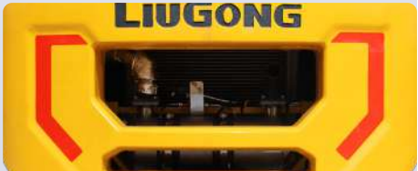
Double-air outlets design • The cooling system is reasonably optimized and adopts aluminum tube and fin fan heaters, independent oil heat dissipation, and large double air outlets , which greatly improves the cooling efficiency, improves the reliability of heavy-duty operation, and ensures the stable operation of key components.
