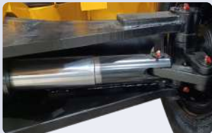
Steering axle • The steering axle angle is increased, the oil cylinder is thickened, and the ordinary bearing is replaced with tapered roller bearing with high reliability, the turning radius is small, and the tire loss is less.
