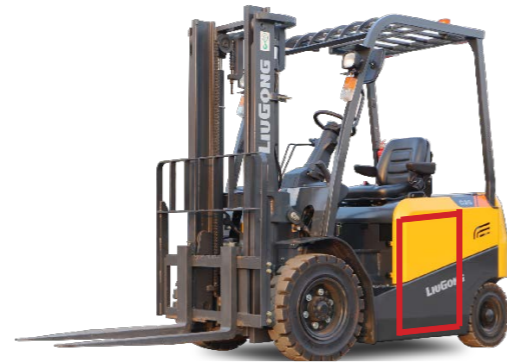
Battery sink down
